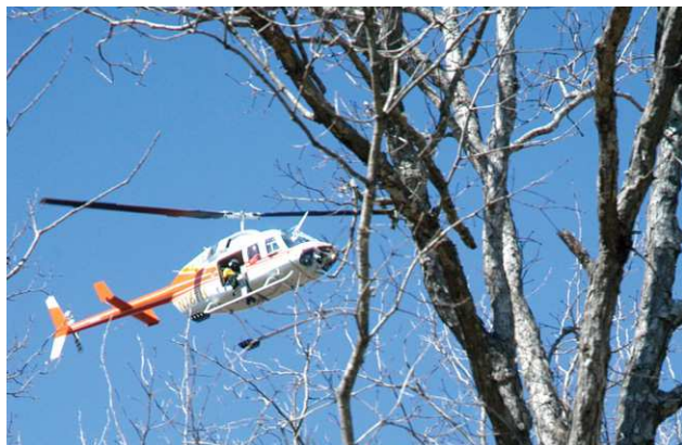
FLYING LOW over the forest with door open, the helicopter drops small plastic balls that catch fire on the ground. On this day, the ship flew over 4,125 acres, dropping some 6,500 balls, one by one. (Quill/Vaughn)
