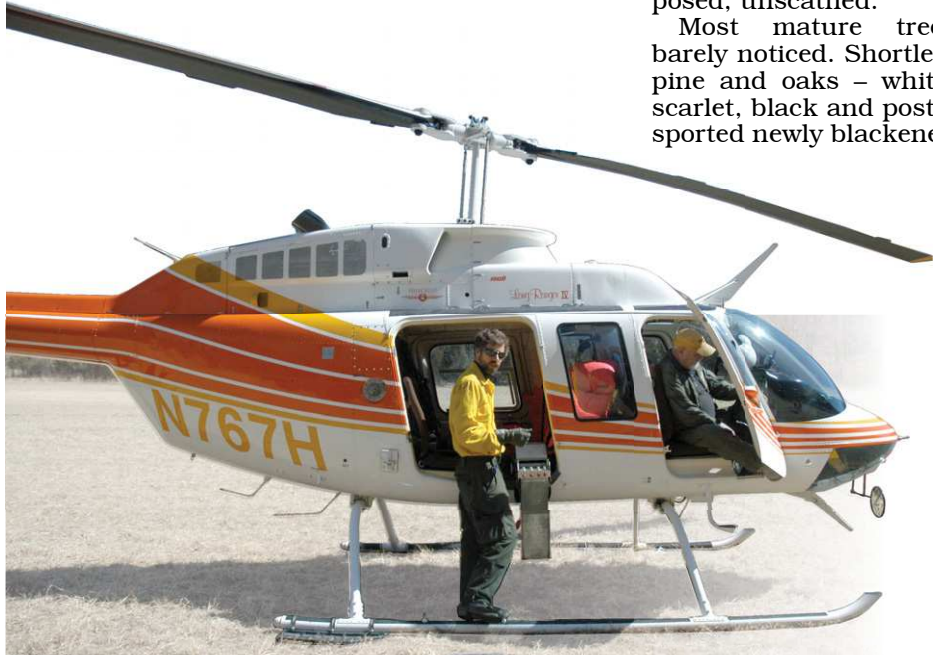
THE SHIP , as they call it, arrived from the Forest Service's main helibase in Rolla and parked in a pasture a few miles from the burn area. Here, pilot Pat Parkhill hits the power-on button so that David Schott, center, can test the Premo machine. That's a device that injects flammable chemicals into spheres like ping-pong balls and then spits them out the chute near Schott's knee. About 20 to 30 seconds after ejection, each ball ignites. (Quill/Vaughn)
